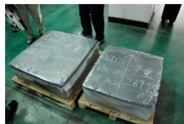
Silicon blocks for the production of solar cells are seen at Yingli Solar in Baoding, China. China's solar manufacturing capacity is currently the largest in the world. ©WWF-China
